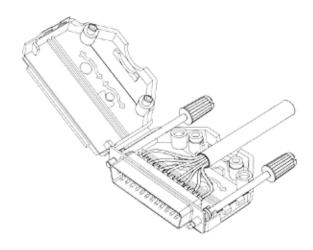
2: Place the connector with mounted cable inside the connector hood together with ferrule. Put the Thumbscrews in place.
