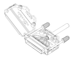
3: Mount the cable clamp and slef-tapping assemblyscrews. Maximum recommended Torque is 0,25Nm.
