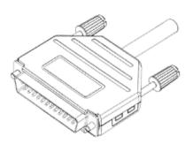
4: Close the connector hood by flipping the top cover into place. Your assembly is ready!
